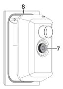
4) Reassemble the coarse separator (5) by putting the edge in the bottom grove (11). Lock with the locking screw (7) and the handle (4).
